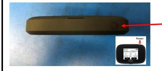
1. Plug the device in to a power outlet and then press the power button on top of the MiFi Box. It is a small gray circle.
